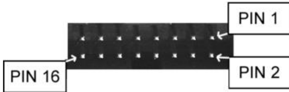
Figure 2-2: MON08 Connector Pin Location
