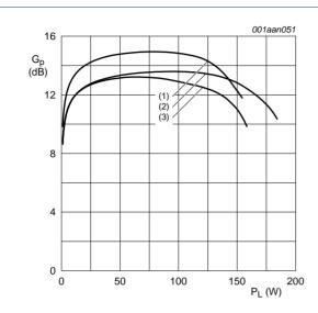
$V_{DS}$  = 32 V;  $I_{Dq}$  = 100 mA;  $t_p$  = 300  $\mu$ s;  $\delta$  = 10 %.
