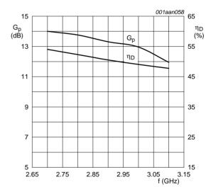
$P_L$  = 130 W;  $V_{DS}$  = 32 V;  $I_{Dq}$  = 100 mA;  $t_p$  = 100  $\mu s;$   $\delta$  = 20 %.
