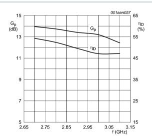
$P_L$  = 130 W;  $V_{DS}$  = 32 V;  $I_{Dq}$  = 100 mA;  $t_p$  = 300  $\mu s;$   $\delta$  = 10 %.
