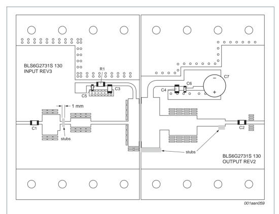
Printed-Circuit Board (PCB): Rogers Duroid 6006; thickness = 0.64 mm;  $\epsilon_r$  = 6.15; thickness of copper plating = 0.035 mm.
