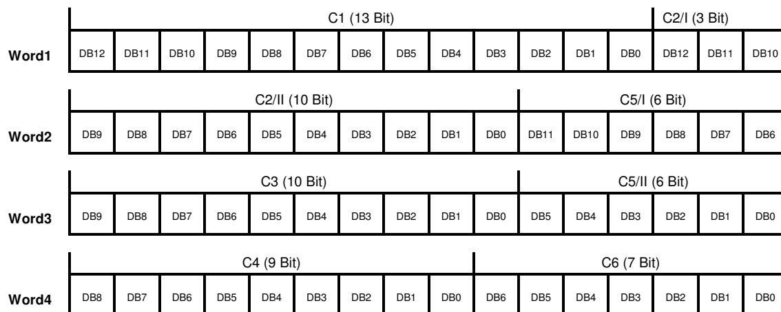
Fig. 4: Arrangement (Bit-pattern) of calibration data in Word1 to Word4.
