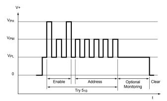
Figure 5. Pulse sequence to provisionally try calibration value 5.
