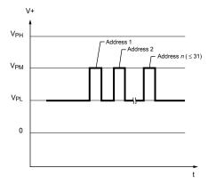
Figure 8. Pulse sequence to select addresses
