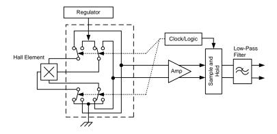
Figure 2. Chopper stabilization circuit (dynamic quadrature offset cancellation)
