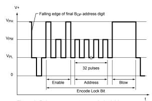
Figure 9. Pulse sequence to encode lock bit
