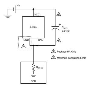
Figure 3. Typical application circuit
