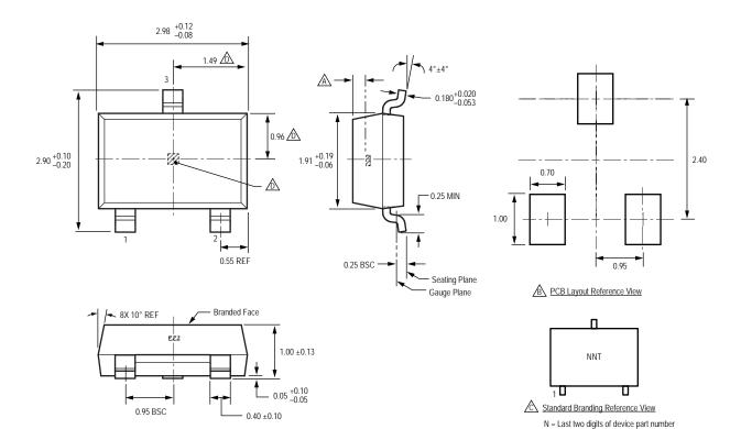
For Reference Only; not for tooling use (reference dwg. 802840) Dimensions in millimeters
