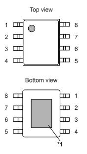
\*1. Connect the heat sink of backside at shadowed area to the board, and set electric potential GND. However, do not use it as the function
