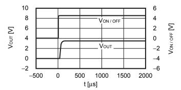
$V_{IN}$  = 3.5 V,  $C_{IN}$  =  $C_L$  = 2.2  $\mu$ F,  $I_{OUT}$  = 100 mA,  $V_{ON\,/\,OFF}$  = 0 V  $\rightarrow$  3.5 V,  $t_r$  = 1.0  $\mu s$ 10 6 VON / OFF 8 4 Von / OFF [V] Vour [V] 6 2 0 4 Vout 2 -2 0 -4 -2 -6 -500 1000 0 500 1500 2000 t [µs]
