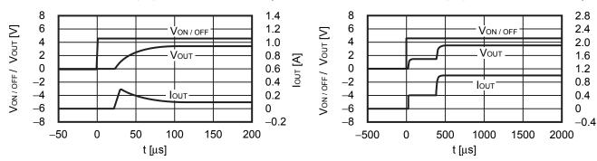
$V_{\text{IN}}$  = 2.0 V,  $C_{\text{IN}}$  =  $C_{\text{L}}$  = 2.2  $\mu$ F,  $C_{\text{SS}}$  = 0 nF,  $I_{\text{OUT}}$  = 1000 mA,  $V_{\text{ON / OFF}}$  = 0 V  $\rightarrow$  2.0 V,  $t_{r}$  = 1.0  $\mu$ s
