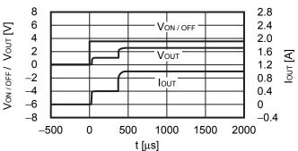
$V_{\text{IN}} = 4.5 \text{ V}, \text{ } C_{\text{IN}} = \text{C}_{\text{L}} = 2.2 \text{ } \mu\text{F}, \text{ } \text{C}_{\text{SS}} = 0 \text{ } \text{nF}, \text{ } \text{I}_{\text{OUT}} = 1000 \text{ } \text{mA}, \\ \text{V}_{\text{ON / OFF}} = 0 \text{ } \text{V} \rightarrow 4.5 \text{ } \text{V}, \text{ } \text{t}_{\text{r}} = 1.0 \text{ } \mu\text{s}$
