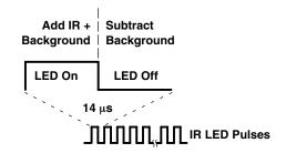
Figure 11. Proximity IR LED Waveform
