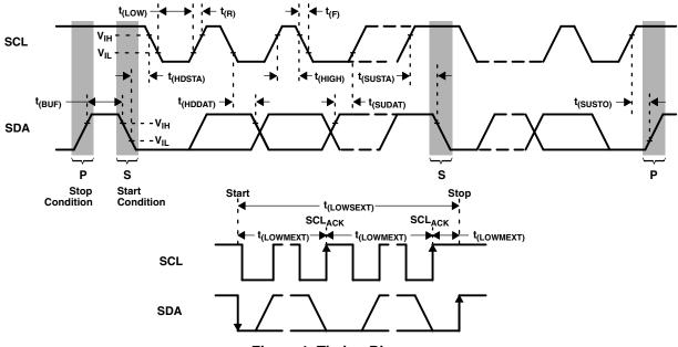
**Figure 1. Timing Diagrams**
