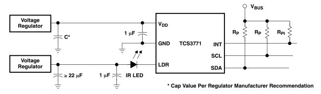
Figure 16. Proximity Sensing Using Separate Power Supplies
