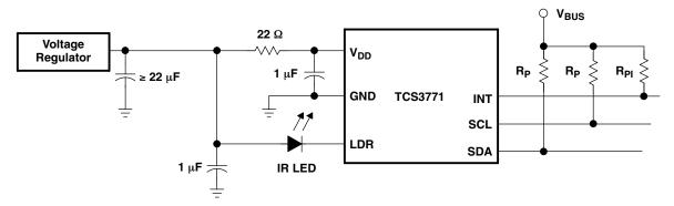
Figure 17. Proximity Sensing Using Single Power Supply
