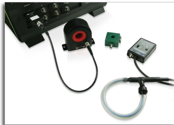
CA10 ProBus current adapter attached to a Danisense Current Transducer. Also shown is a Pearson Current Transformer and a PEM-UK Rogowski Coil, which are also third party devices that can be used with the CA10.
