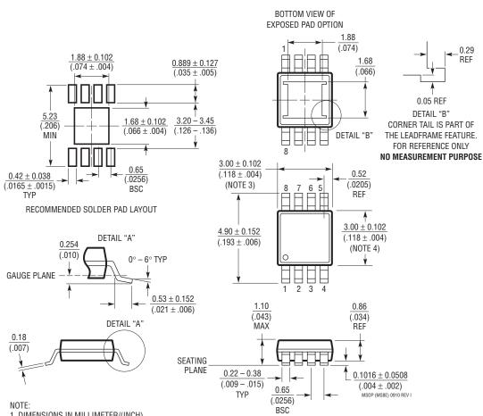
**MS8E** Package 8-Lead Plastic MSOP, Exposed Die Pad (Reference LTC DWG # 05-08-1662 Rev I)
