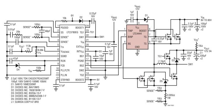
LTC3780 High Efficiency 8V to 80V  $V_{\rm IN}$  to 12V/5A Buck-Boost DC/DC Converter
