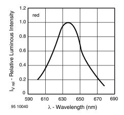
Fig. 7 - Relative Intensity vs. Wavelength
