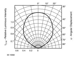
Fig. 2 - Relative Luminous Intensity vs. Angular Displacement
