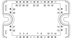
All multiple inputs and outputs must be shorted together Example: 13/14 ; 29/30 ; 22/23 ...
