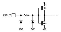
Figure 7. Input Equivalent Circuit
