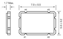
Figure 1) CSM-8 - Side and Top view
