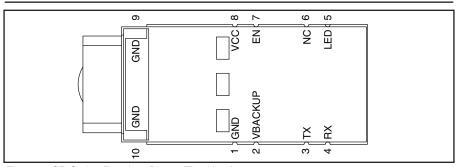
Figure 2: SR Series Receiver Pinout (Top View)
