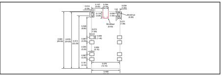
Figure 7: Recommended PCB Layout
