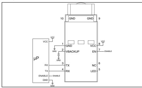
Figure 3: SR Series Module Typical Application
