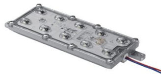
(b) Module without Fin [Thermal management by Fixture]
