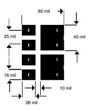
FIGURE 2. Footprint With Copper Spreading
