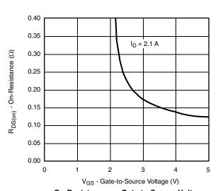
On-Resistance vs. Gate-to-Source Voltage
