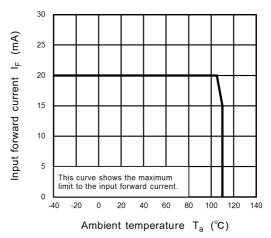
Fig. 13.2.2 I<sub>F</sub> - T<sub>a</sub>
