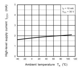
Fig. 13.2.6 I<sub>CCH</sub> - T<sub>a</sub>
