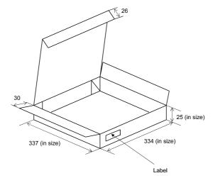
Fig. 18.4.1 1 reel/carton (unit: mm)
