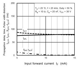
Fig. 13.2.12  $t_{pLH}, t_{pHL}, |t_{pHL}-t_{pLH}| - I_F$
