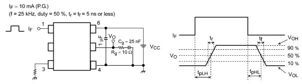
Fig. 13.1.7 Switching Time Test Circuit and Waveform
