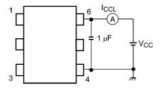
Fig. 13.1.6 I<sub>CCL</sub> Test Circuit
