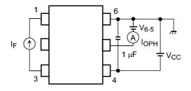
Fig. 13.1.1 I<sub>OPH</sub> Test Circuit
