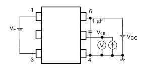
Fig. 13.1.4 V<sub>OL</sub> Test Circuit
