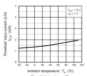
Fig. 13.2.4 I<sub>FLH</sub> - T<sub>a</sub>
