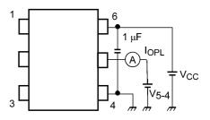
Fig. 13.1.2 I<sub>OPL</sub> Test Circuit
