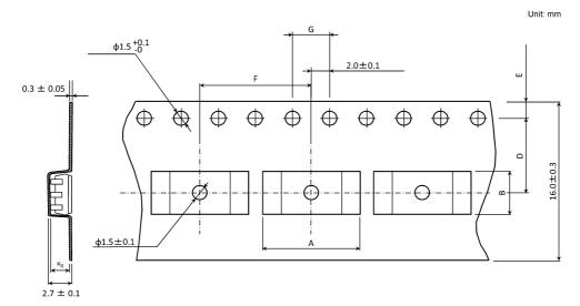
Table Tape Dimensions (unit: mm, tolerance: ±0.1)
