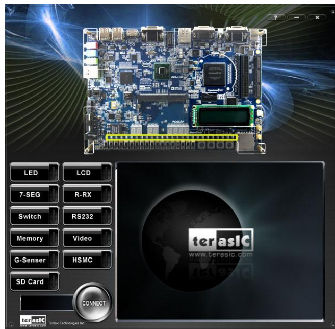
Figure 2-1 The DE2i-150 Control Panel
