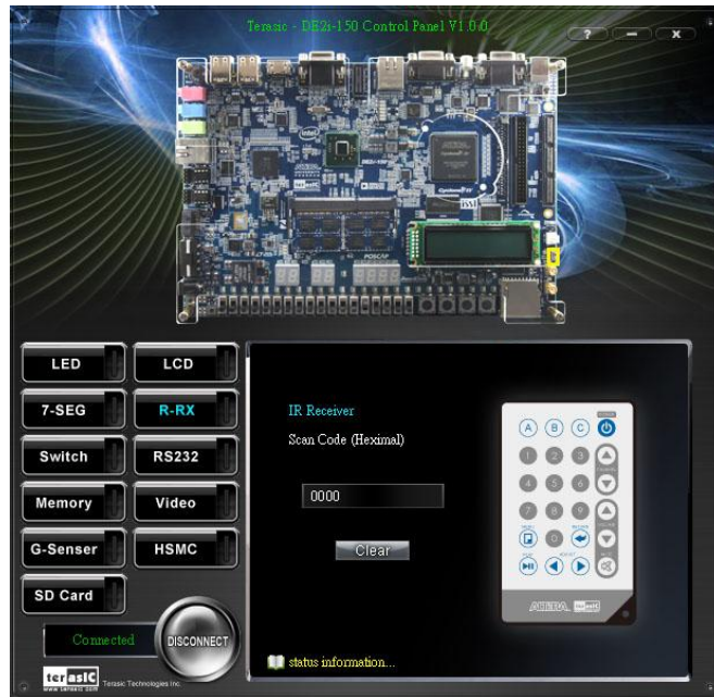
Figure 2-12 Testing the IR receiver using remote controller
