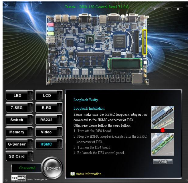
Figure 2-11 HSMC loopback verification test performed under Control Panel
