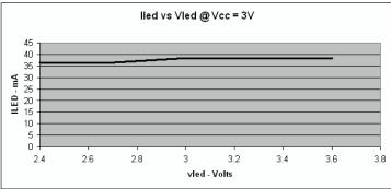
Figure 2. LED current vs. VLED.
