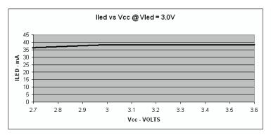
Figure 1. LED current vs. Vcc.
