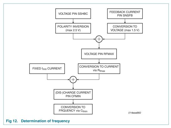
Two external components determine the frequency range:
