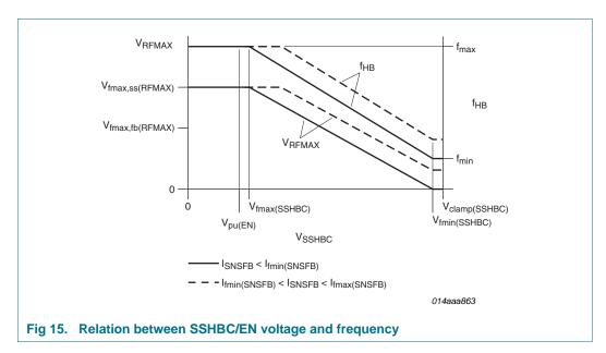
$V_{RFMAX}$  and  $V_{SSHBC/EN}$  are of opposite polarity. At initial start-up,  $V_{SSHBC/EN}$  is below  $V_{fmax(SSHBC)}$  (typ. 3.2 V), which corresponds to the maximum frequency. During start-up,  $C_{ss(HBC)}$  is charged,  $V_{SSHBC/EN}$  rises and the frequency decreases. The contribution of the soft start function is zero when  $V_{SSHBC/EN}$  is above  $V_{fmin(SSHBC)}$  (typ. 7.9 V).
