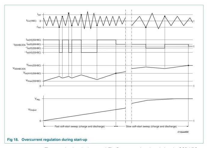
The protection timer is also started. The Restart state is activated when the OCR-HBC condition is still present after the protection time has elapsed.
