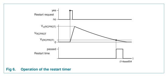
Figure 6 shows the operation of the restart timer. Normally  $C_{prot}$  is discharged to 0 V. When a restart is requested,  $C_{prot}$  is quickly charged to the upper switching level  $V_{u(RCPROT)}$ . Then the RCPROT pin becomes high ohmic and  $C_{prot}$  discharges through  $R_{prot}$ . The restart time has elapsed when  $V_{RCPROT}$  reaches the lower switching level  $V_{l(RCPROT)}$  (typ. 0.5 V). The IC then restarts and  $C_{prot}$  is discharged.
