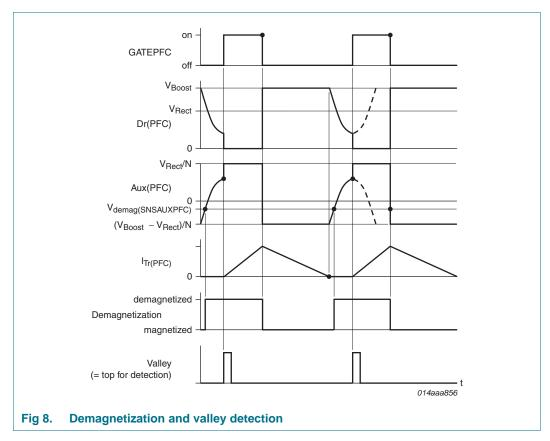
Valleys are detected by the valley sensing block connected to the SNSAUXPFC pin. This block measures the voltage at the auxiliary winding of the PFC transformer, which is a reduced and inverted copy of the MOSFET drain voltage. When a valley of the drain voltage (= top at SNSAUXPFC voltage) is detected, the MOSFET is switched on.
