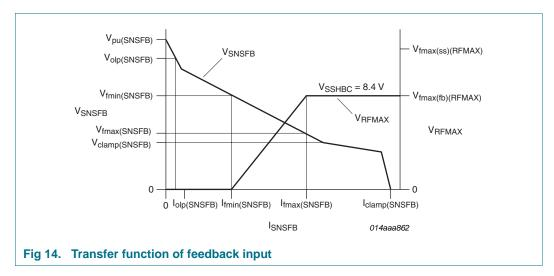
Below the level for minimum frequency,  $V_{SNSFB}$  is clamped at  $V_{clamp(SNSFB)}$  (typ. 3.2 V). This clamp enables a fast recovery of the output voltage regulation loop after an overshoot of the output voltage. The maximum current the clamp can deliver is  $I_{clamp(SNSFB)}$  (typ. 7.3 mA).
