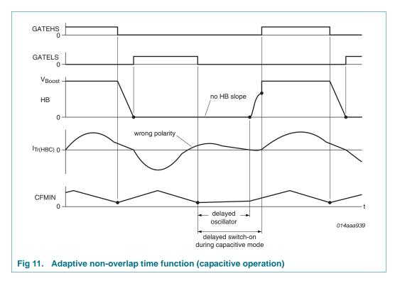
The MOSFET will be forced to switch on if the half-bridge slope fails to start and the oscillator voltage reaches  $V_{u(CFMIN)}$ .
