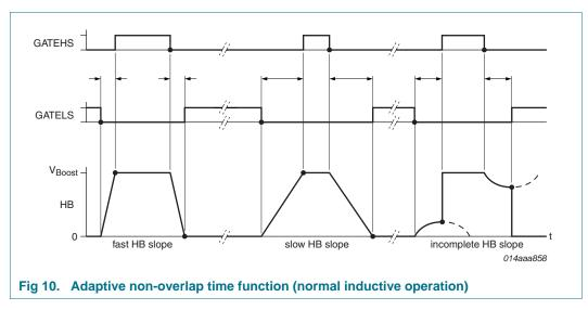
The non-overlap time depends on the HB slope, but has upper and lower limits.
