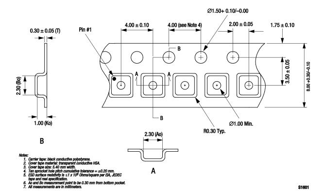
Figure 6. SMP1325-087LF Tape and Reel Dimensions
