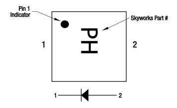
Figure 4. Typical Case Markings (Top View)
