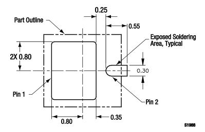
Figure 3. SKY1325-087LF PCB Layout Footprint (Top View)
