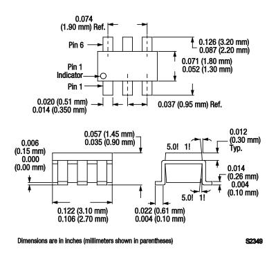
Figure 10. PD18-73/PD18-73LF 6-Pin SOT-6 Package Dimensions
