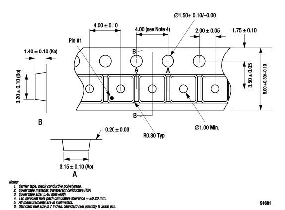
Figure 11. PD18-73/PD18-73LF Tape and Reel Dimensions
