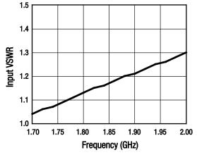
Figure 7. Input VSWR vs Frequency
