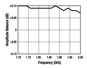
**Figure 6. Amplitude Balance vs Frequency**
