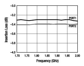
**Figure 3. Insertion Loss vs Frequency**
