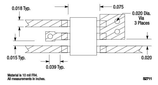
Figure 9. PD18-73/PD18-73LF Recommended Board Layout
