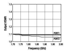
**Figure 4. Output VSWR vs Frequency**
