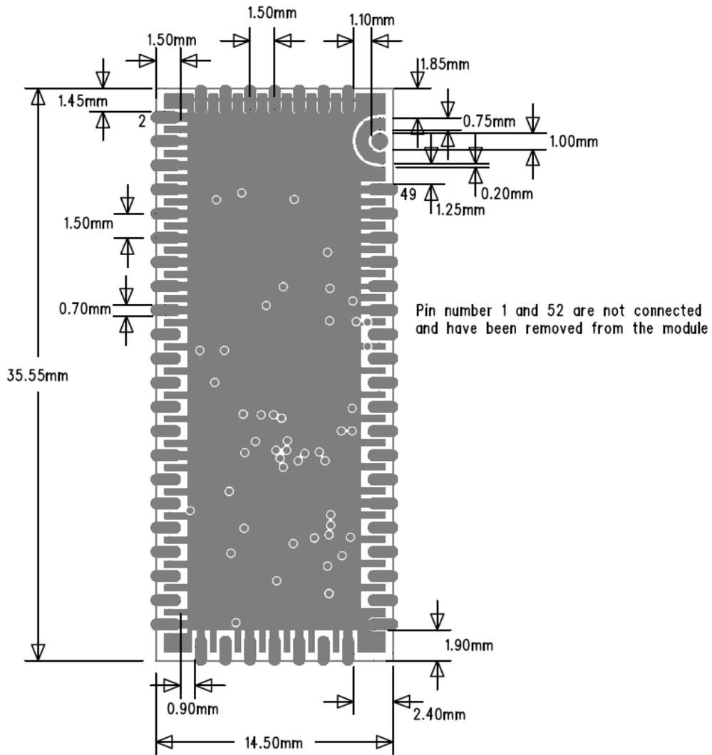
Figure 4: Physical dimensions (top view)
