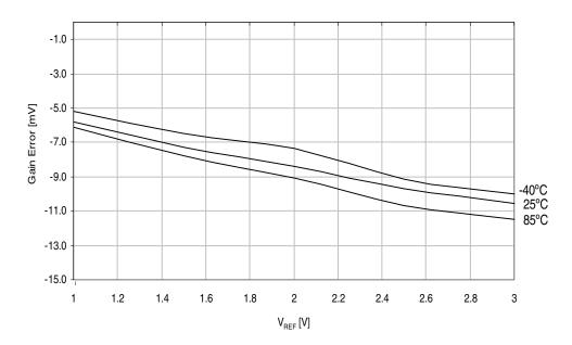
Figure 37-33.ADC Gain Error vs. V<sub>REF</sub>.
