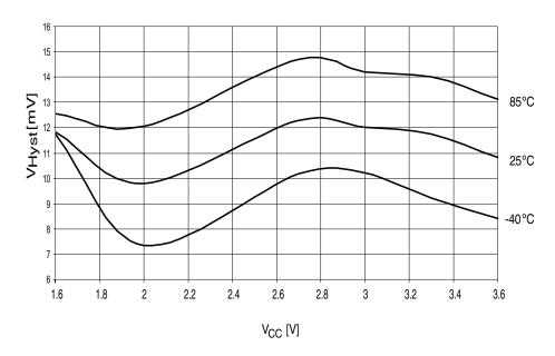
Figure 37-39. Analog comparator hysteresis vs. V<sub>CC</sub>. *High-speed mode, large hysteresis*.
