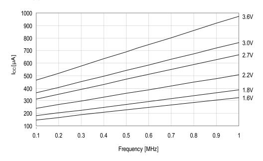
Figure 37-2. Active supply current vs. frequency.  $f_{SYS} = 1 - 32MHz$  external clock,  $T = 25^{\circ}C$ .
