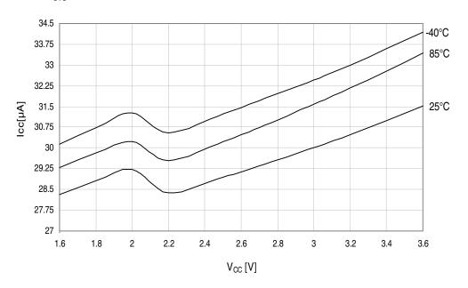
Figure 37-8. Idle mode supply current vs.  $V_{CC}$ .  $f_{SYS} = 2MHz$  internal oscillator.
