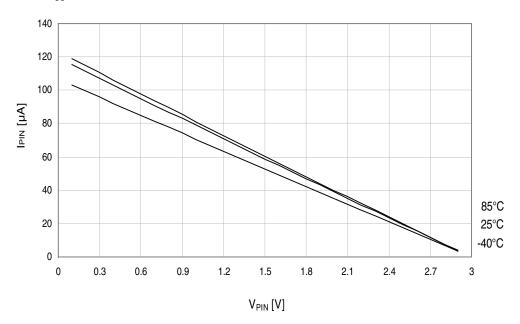
Figure 37-14.I/O pin pull-up resistor current vs. pin voltage.
