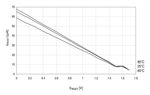
Figure 37-53.Reset pin pull-up resistor current vs. reset pin voltage.
