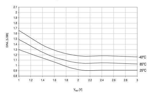
Figure 37-27.ADC DNL vs.  $V_{REF}$ . SE Unsigned mode,  $V_{CC}$  = 3.6V, external reference.
