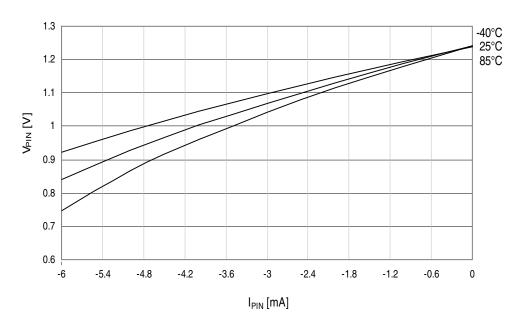
Figure 37-16.I/O pin output voltage vs. source current.
