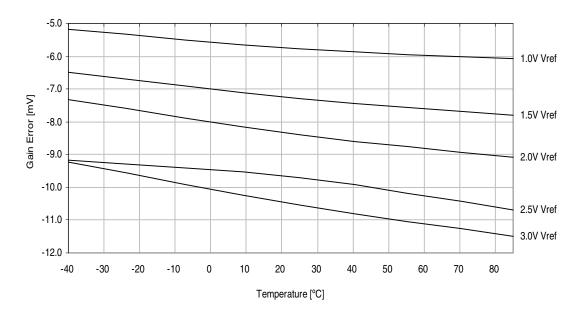
Figure 37-37.ADC Gain Error vs. Temperature. SE Unsigned mode,  $V_{CC} = 3.6V$ , external reference.
