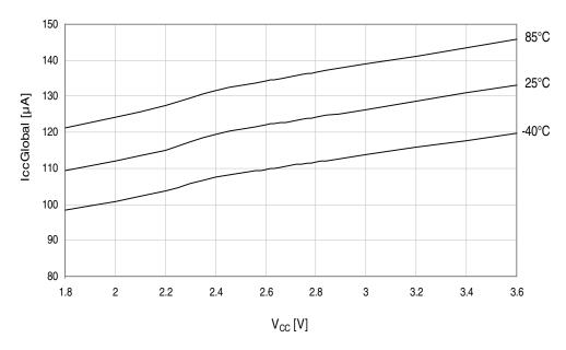
Figure 37-47.BOD current consumption vs.  $V_{CC}$ . Sampled mode, BOD level = 1.6V.
