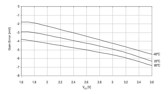
Figure 37-36.ADC Gain Error vs. Temperature.
