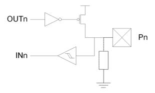
Figure 15-6. I/O configuration - Wired-AND with optional pull-up
