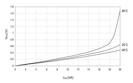
Figure 37-19.I/O pin output voltage vs. sink current.
