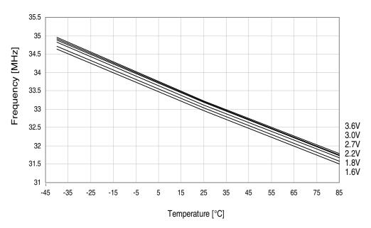
Figure 37-66.32MHz internal oscillator frequency vs. temperature.
