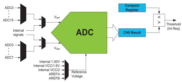
The ADC may be configured for 8- or 12-bit result, reducing the minimum conversion time (propagation delay) from 3.35µs for 12-bit to 2.3µs for 8-bit result.
