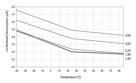
Figure 37-83.Psave vs. Temperature *RTC, WDT, BOD sampled.*
