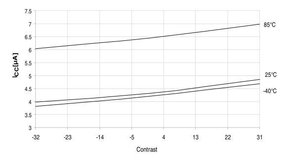
Figure 37-81.Psave LCD LP 32Hz vs. Temperature
