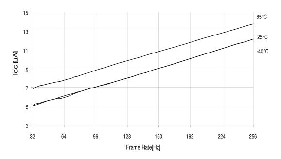
Figure 37-79. $I_{CC}$  vs. Contrast 32Hz Low Power Frame Rate from 32.768KHz TOSC, w/o pixel load,  $V_{CC}$  = 1.8V
