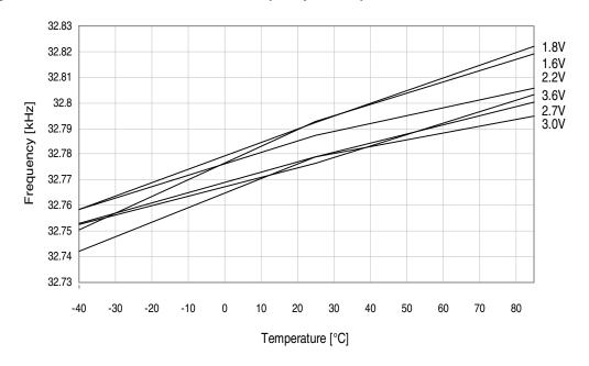
Figure 37-58.32.768kHz ULP internal oscillator frequency vs. temperature.
