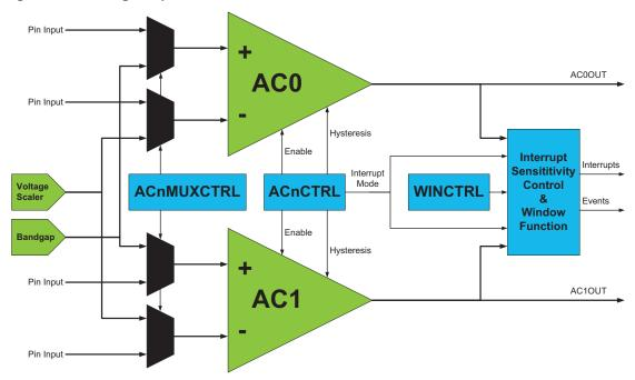
The window function is realized by connecting the external inputs of the two analog comparators in a pair as shown in Figure 30-2.
