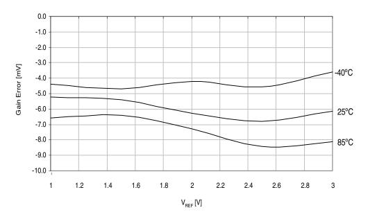
Figure 37-34.ADC Gain Error vs. V<sub>CC</sub>.
