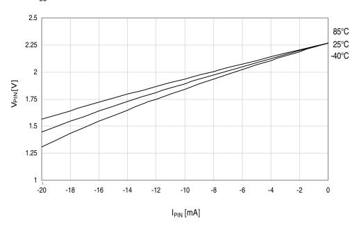
Figure 37-18.I/O pin output voltage vs. sink current.
