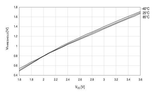
Figure 37-56.Reset pin input threshold voltage vs.  $V_{CC.}$   $V_{IL}$  - Reset pin read as "0".
