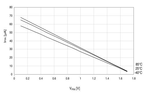
Figure 37-13.I/O pin pull-up resistor current vs. input voltage.
