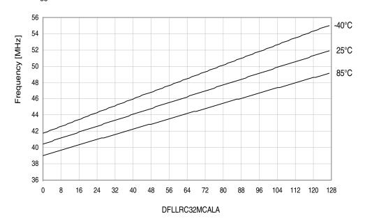
Figure 37-70.32MHz internal oscillator frequency vs. CALB calibration value.  $V_{CC}$  = 3.0V, DFLL enabled.
