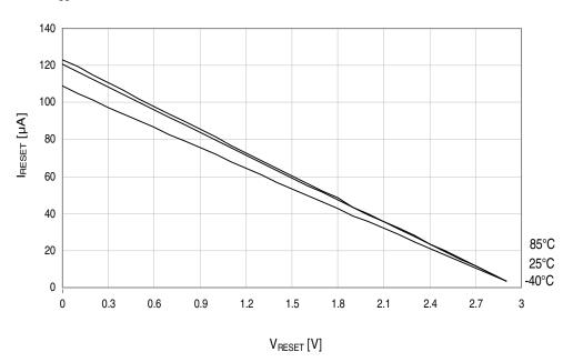
Figure 37-54.Reset pin pull-up resistor current vs. reset pin voltage.
