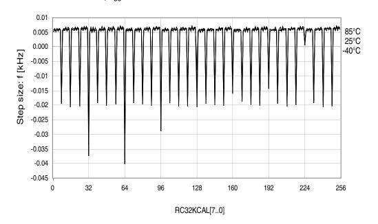
Figure 37-60.32.768kHz internal oscillator frequency vs. calibration value.  $V_{CC} = 3.0V, T = 25$ °C.
