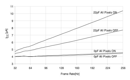
Figure 37-77. $I_{CC}$  vs. Frame Rate 32Hz Low Power Frame Rate from 32.768KHz TOSC, w/ and w/o pixel load,  $V_{CC}$  = 3.0V, T = 25°C
