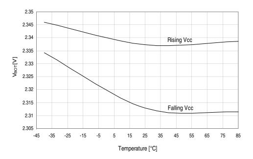
Figure 37-50.BOD thresholds vs. temperature. BOD level = 3.0V.
