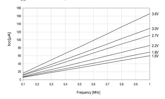
Figure 37-6. Idle mode supply current vs. frequency.  $f_{SYS} = 1 - 32MHz$  external clock, T = 25°C.
