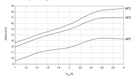
Figure 37-30.ADC Offset vs.  $V_{REF}$ .
