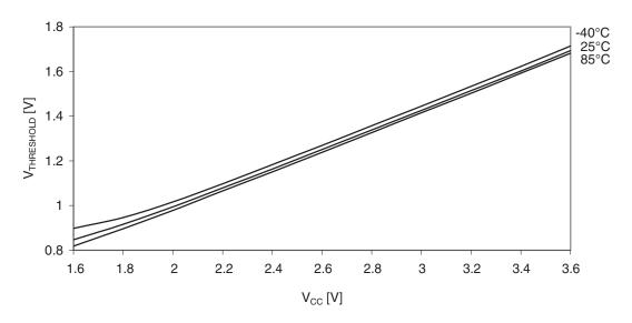
Figure 37-22.I/O pin input threshold voltage vs.  $V_{CC}$ .  $V_{IL}$  I/O pin read as "0".
