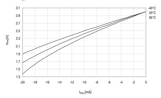
Figure 37-17.I/O pin output voltage vs. source current.
