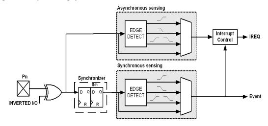
When a pin is configured with inverted I/O, the pin value is inverted before the input sensing.
