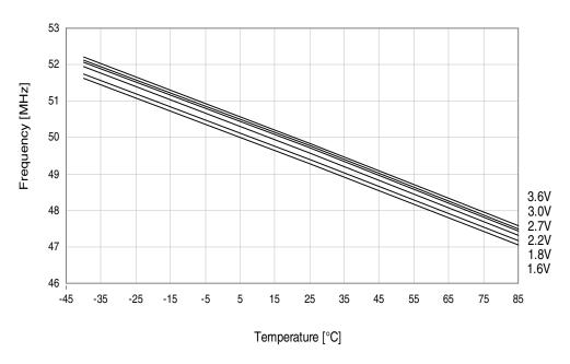
Figure 37-72. 48MHz internal oscillator frequency vs. temperature.
