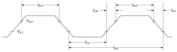
Table 36-25. External clock used as system clock without prescaling.
