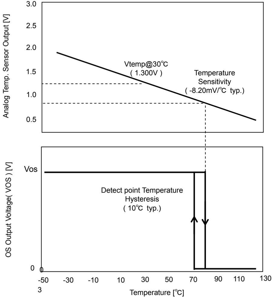
If the temperature over detect temperature, internal comparator operate OS output “H” to “L”.(ex.active “L” Type)
