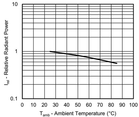
Fig. 6 - Relative Radiant Power vs. Ambient Temperature
