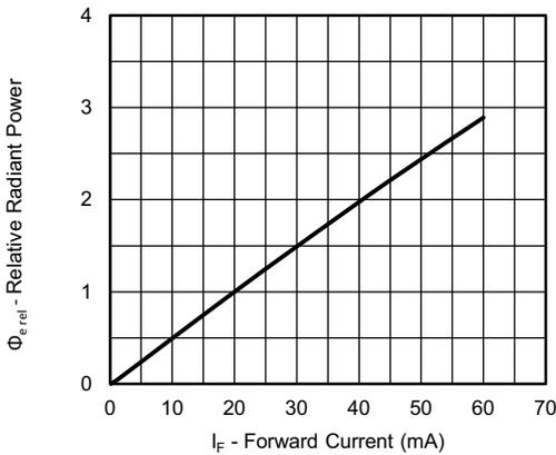
Fig. 2 - Relative Radiant Power vs. Forward Current
