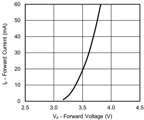
Fig. 3 - Forward Current vs. Forward Voltage
