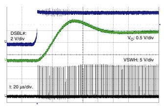
Enable with  $V_{IN}$  = 12 V,  $V_{OUT}$  = 1.2 V,  $F_S$  = 500 kHz
