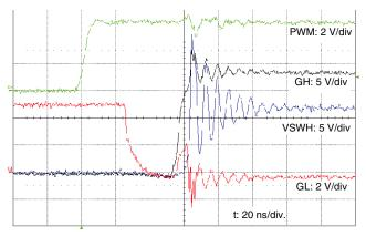
Switching Waveforms at PWM rising edge  $\rm V_{IN}=12~V,\,V_{OUT}=1.2~V,\,F_{S}=500~kHz,\,I_{OUT}=30~A$
