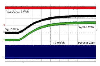
Startup with  $V_{IN}$  ramping up  $V_{IN}$  = 12 V,  $V_{OUT}$  = 1.2 V,  $F_S$  = 500 kHz
