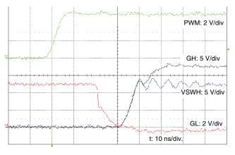
Switching Waveforms at PWM rising edge  $V_{IN}$  = 12 V,  $V_{OUT}$  = 1.2 V,  $F_S$  = 500 kHz,  $I_{OUT}$  = 0 A
