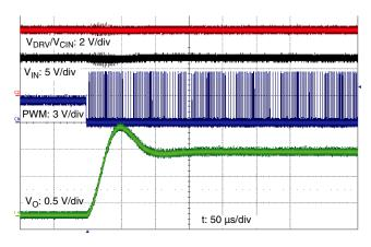
PWM Start with  $V_{IN}$  = 12 V,  $V_{OUT}$  = 1.2 V,  $F_S$  = 500 kHz
