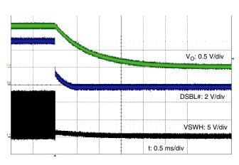
Disable with  $V_{IN}$  = 12 V,  $V_{OUT}$  = 1.2 V,  $F_{S}$  = 500 kHz
