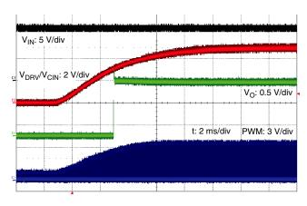
Startup with  $V_{DRV}/V_{CIN}$  ramping up  $V_{IN}$  = 12 V,  $V_{OUT}$  = 1.2 V,  $F_{S}$  = 500 kHz
