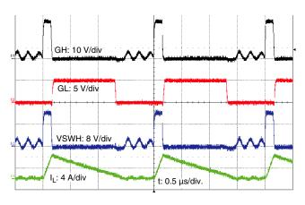
Switching Waveforms with SMOD enabled  $\rm V_{IN}$  = 12 V,  $\rm V_{OUT}$  = 1.2 V,  $\rm F_{S}$  = 500 kHz,  $\rm I_{OUT}$  = 1.5 A
