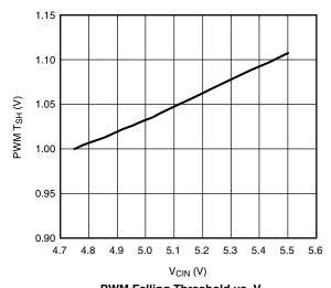
PWM Falling Threshold vs.  $V_{CIN}$
