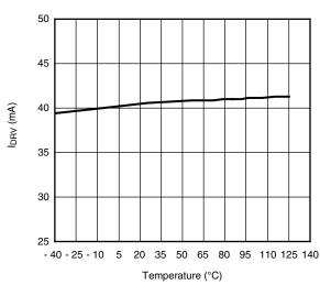
$I_{DRV}$  (mA) vs. Temperature at Frequency = 1 MHz D = 10 %,  $V_{CIN}$  =  $V_{DRV}$  = 5 V
