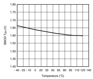
SMOD Rising Threshold (V) vs. Temperature (°C) V<sub>CIN</sub> = V<sub>DRV</sub> = 5 V
