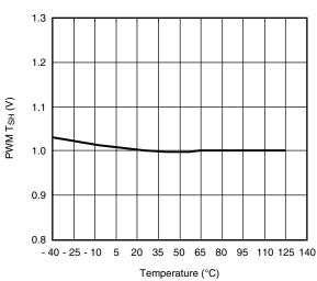
PWM Falling Threshold (V) vs. Temperature (°C)  $V_{CIN} = V_{DRV} = 5 \text{ V}$
