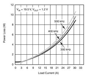
$V_{IN}$  = 12 V and 19.5 V,  $V_{OUT}$  = 1.2 V,  $V_{DRV}$  =  $V_{CIN}$  = 5 V; No Air Flow IHLP5050FDERR33M01 Inductor L = 330 nH, DER = 0.83  $m\Omega$
