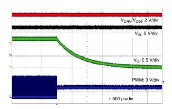
PWM Turn-off with  $V_{IN}$  = 12 V,  $V_{OUT}$  = 1.2 V,  $F_S$  = 500 kHz
