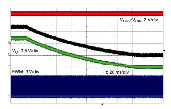
Power Off with  $V_{IN}$  ramping down  $V_{IN}$  = 12 V,  $V_{OUT}$  = 1.2 V,  $F_{S}$  = 500 kHz
