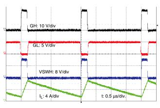
Switching Waveforms with SMOD disabled  $V_{IN}$  = 12 V,  $V_{OUT}$  = 1.2 V,  $F_S$  = 500 kHz,  $I_{OUT}$  = 4 A
