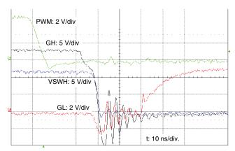
Switching Waveforms at PWM falling edge  $\rm V_{IN}=12~V,\,V_{OUT}=1.2~V,\,F_{S}=500~kHz,\,I_{OUT}=30~A$
