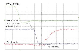
Switching Waveforms at PWM falling edge  $V_{IN}$  = 12 V,  $V_{OUT}$  = 1.2 V,  $F_{S}$  = 500 kHz,  $I_{OUT}$  = 0 A
