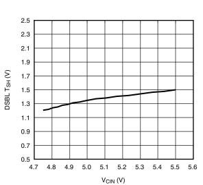
SMOD Falling Threshold vs.  $V_{\rm CIN}$
