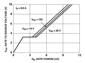
Figure 7. Gate Charge Characteristics
