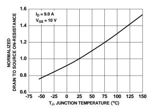
Figure 3. Normalized On-Resistance vs Junction Temperature
