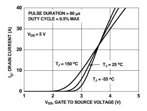
Figure 5. Transfer Characteristics
