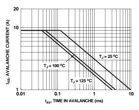
Figure 9. Unclamped Inductive Switching Capability
