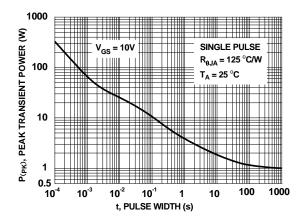
Figure 12. Single Pulse Maximum Power Dissipation
