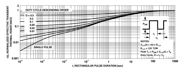
Figure 13. Transient Thermal Response Curve
