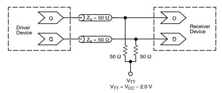
Figure 6. Typical Termination for Output Driver and Device Evaluation (See Application Note AND8020/D – Termination of ECL Logic Devices.)
