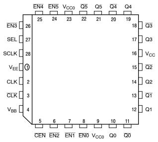
\*All  $V_{CC}$  and  $V_{CCO}$  pins are tied together on the die.
