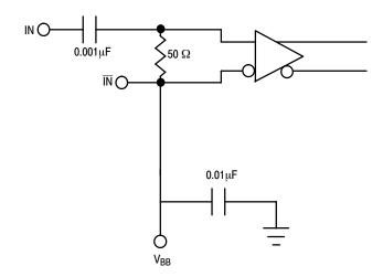
Figure 4. AC Coupled Input
