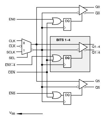
Figure 2. Logic Diagram
