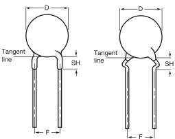
Capacitors with 10 mm (0.40") lead spacing
