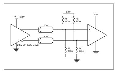
Figure 2A. 2.5V LVPECL Driver Termination Example
