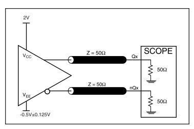
2.5V LVPECL Output Load AC Test Circuit
