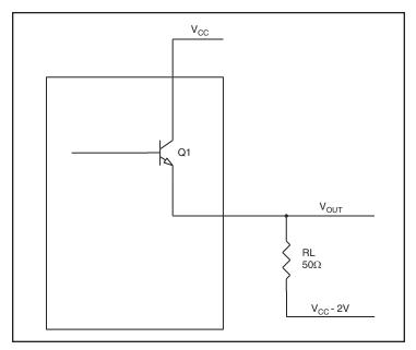
Figure 3. LVPECL Driver Circuit and Termination
