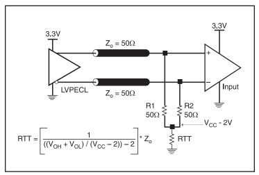
Figure 1A. 3.3V LVPECL Output Termination
