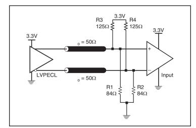
Figure 1B. 3.3V LVPECL Output Termination
