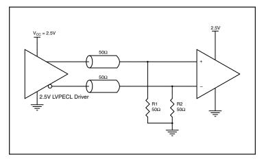
Figure 2C. 2.5V LVPECL Driver Termination Example
