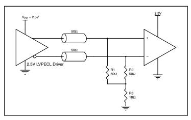
Figure 2B. 2.5V LVPECL Driver Termination Example
