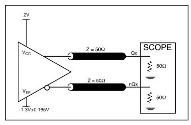
3.3V LVPECL Output Load AC Test Circuit
